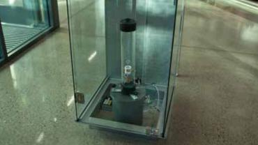
Whenever fault lines shift, library patrons in the PSC will be among the first to know about it. The slinky seismometer uses electromagnetic induction to detect ground motion; it is sensitive enough to register a 6.0 earthquake occurring anywhere in the world.
